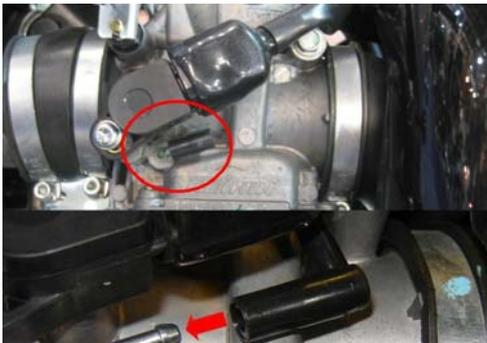
On some models there are spare vacuum points, these might be redundant in certain markets due to emissions laws or might exist to facilitate carburettor / throttle body balancing.
