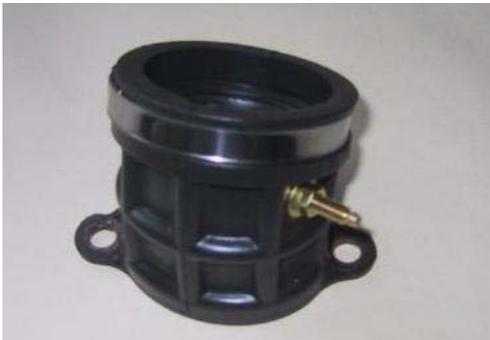
Where no vacuum points or pipes exist it is still possible to access vacuum. To do so it is necessary to drill the inlet manifold or carburettor and install the Scottoilier Universal Spigot, this is available on request.
