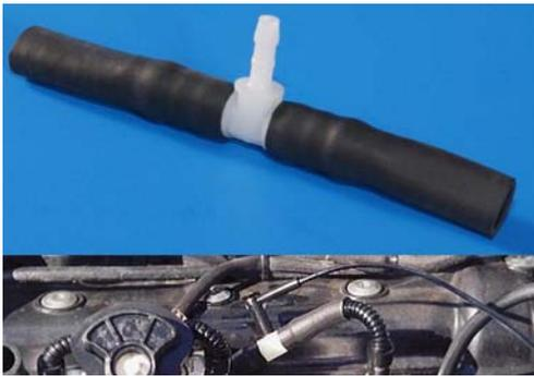
Some Triumph models, particularly 955cc variants, have corrugated vacuum pipes from each throttle body. In order to make use of these, without compromising the air tight system, Scottoilier can supply a special T-Piece with Viton rubber sleeves which seal on the outside of the corrugated pipes.
