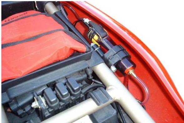
The Reservoir Clamp has been used here to mount the reservoir on the sub frame behind a side panel. The clamp is secured to an existing M6 bolt.
