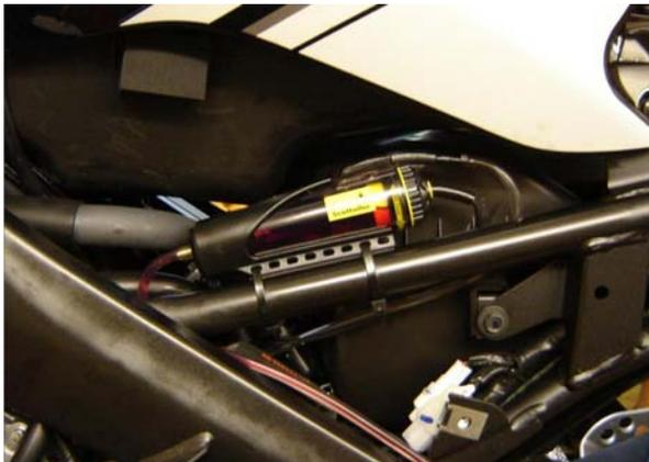
Scottoiler have designed a Reservoir Cage which provides a more sophisticated fitting option for tubular frame members. Using cable ties more discretely to secure the reservoir.
