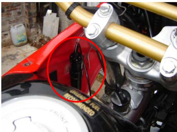
Reservoir mounted behind a front side panel secured using Instant Adhesive and Reservoir Mounting Sleeve.
