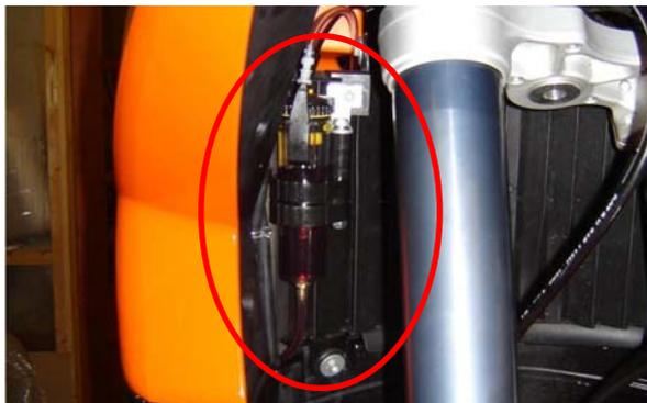
It is sometimes possible to secure the reservoir to the radiator protective louvers.
