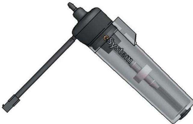
The Scottoiler eSystem uses an electro magnetic piston pump to deliver oil at a user determined rate, independent of gravity head and temperature.
