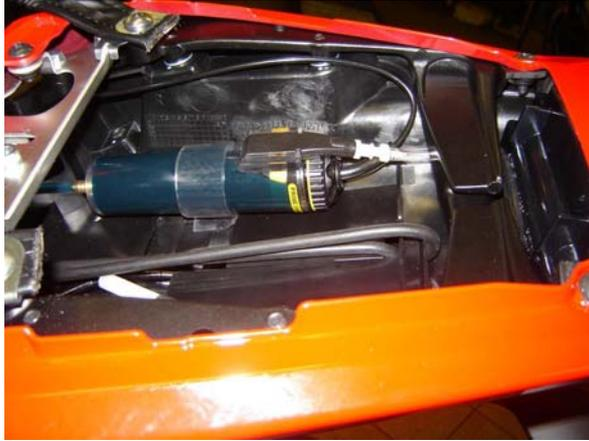
To mount on a square section tube or a flat surface without the need for drilling, the reservoir can be inserted into the mounting sleeves provided.
