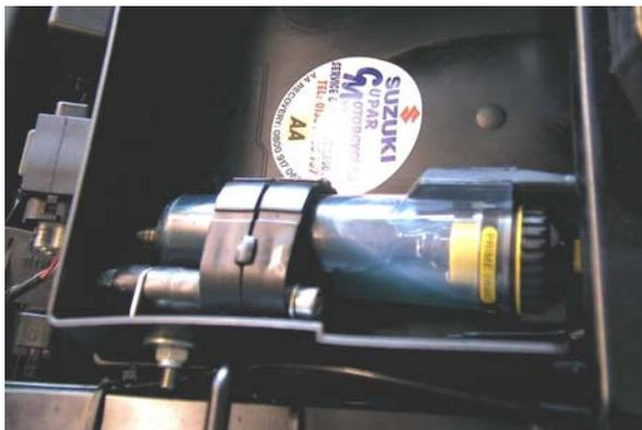
In this picture a 6.2mm hole has been drilled in the plastic under the seat and the Reservoir Clamp has been secured to this hole using washers and an M6 nut.
