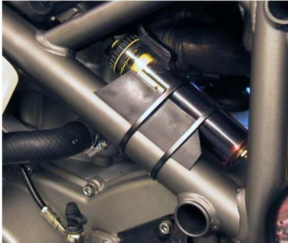
The cradle is supplied to allow fitting to tubular frame members. Position the reservoir in the short side of the cradle and then fit the cradle to a frame member, secure using the cable ties provided.
