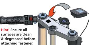
**Bracket Mount.** Fits to any existing M5/M6 bolt. Fit display unit to bracket (part 5) using M3 screws (part 16).
