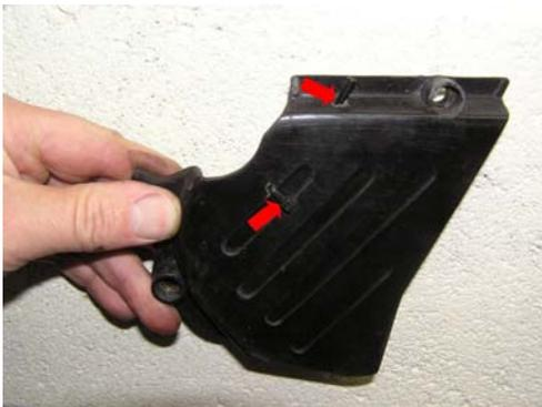
The picture opposite highlights where 3 holes have been drilled in the sprocket cover. The hole in the top is where the vacuum tubing enters the front sprocket cover and should be 3.2 to 3.5mm in diameter to give a good fit for the black vacuum tubing.
