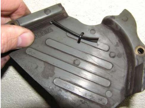
It is possible to adapt the OEM Ducati Front Sprocket cover to incorporate a Scottoil front sprocket feed. This is recommended on models with complex single sided swinging arms.
