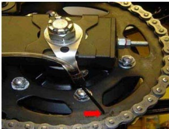
The Dispenser Plate is designed to be secured on the rear wheel spindle, as shown opposite.
