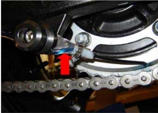
The **Small Dispenser Plate** is used in the same way to secure the nib and is ideal for mounting on Paddock Stand bobbin bosses or chain / sprocket guard mounting bolts.
