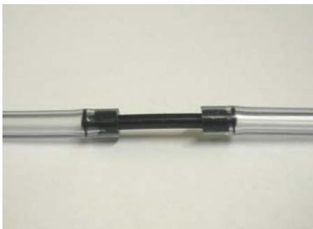
If making a joining piece, repeat the above steps to mushroom the other end of the black nylon tube and connect the new section of delivery tubing.
