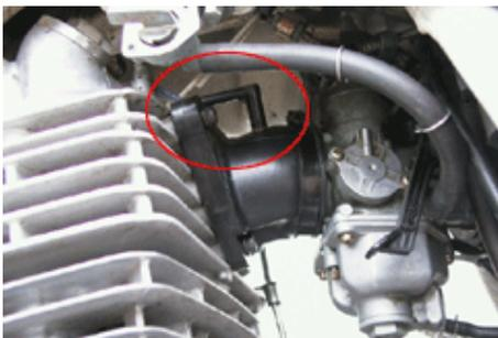
For bikes with **single carburetors**, it is necessary to drill the inlet tract. This can be quite straightforward if the rubber manifold between the cylinder head and the carburetor is long enough to accept the m5 or m6 spigot supplied in the kit.
