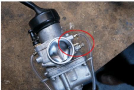
Drill a 4.2mm hole and cut an M5 thread for M5 spigot (5.2mm hole and M6 thread for M6 spigot). **Ensure there are no metal particles on the carburetor or throttle body before re-assembly.**
