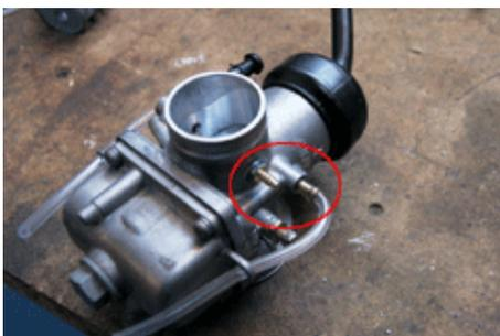
Insert the spigot, using a washer and thread lock or silicon in the threads to ensure an airtight seal. Carefully install the throttle body or carburetor onto the engine and push the vacuum damper onto the spigot. Route the vacuum tubing neatly to your chosen RMV position.
