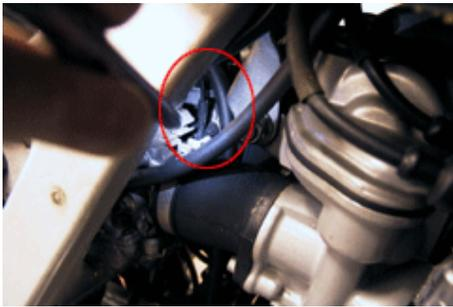
Some single cylinder motorcycles have twin carbs. This includes pre fuel injected **BMW F650's**, and some **Aprilia Pegasos**. Single cylinders with twin carbs have a vacuum point to balance the carbs. Picture of bung is shown left, and balance pipe shown below left on a 4 carb model. Twin carbs can have the same.
