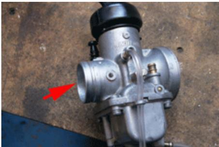
It is best to use the M5 spigot (the M6 spigot can be used should there be any problems with the M5). Always cover the open inlet on the cylinder head with a clean cloth to avoid the risk of contamination. Before drilling the hole make sure it is in the correct position, and the spigot and vacuum damper (or vacuum tubing) do not touch the throttle cables or mechanism when the parts are re-assembled on the engine.
