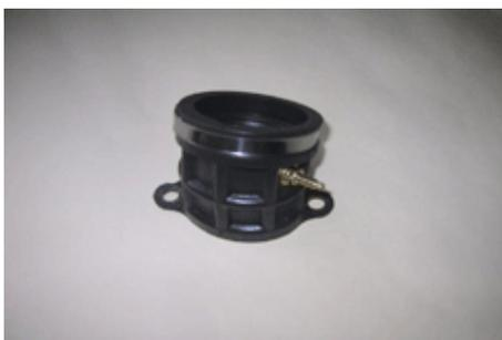
Remove the rubber inlet manifold. Drill a 4mm hole in the inlet manifold, being careful to remove any swarf created. Fit the M5 spigot from the Scottoil kit, using a silicon type sealer to ensure an airtight seal, and washers supplied in the kit, as shown left.
